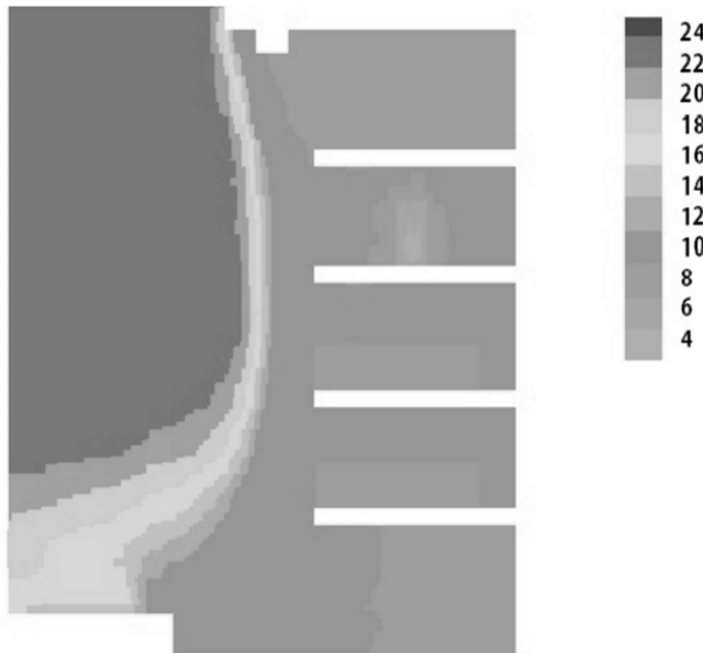
Fig. 5. Simulation of cabinet temperature field in defrost cycle (case 1)
